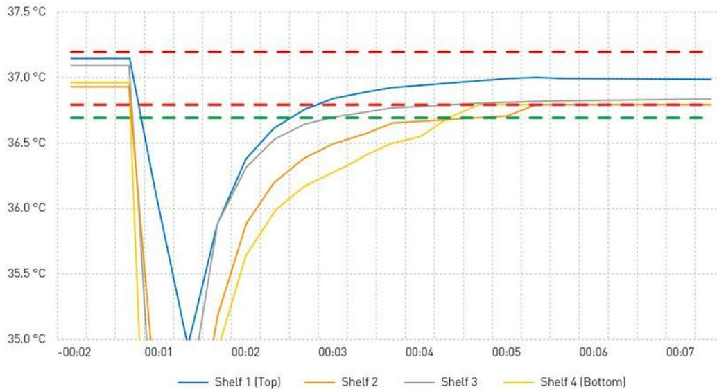
**Temperature recovery test:** Incubator set point 37°C; Temperature probes: 9 probes/shelf; Room temperature: 21°C; Door opening: 15 seconds. Green dashed line represents nominal uniformity (+/- 0.3°C from set point); Red dashed line is +/- 0.2°C from set point.
